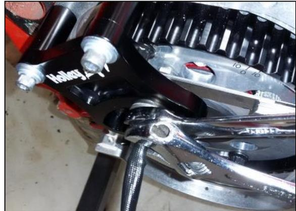
Figure 15: Locking Sensor Gap & Position
