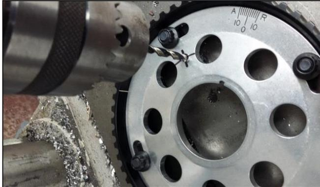
**Figure 11: Drilling the Cam Hub.**
