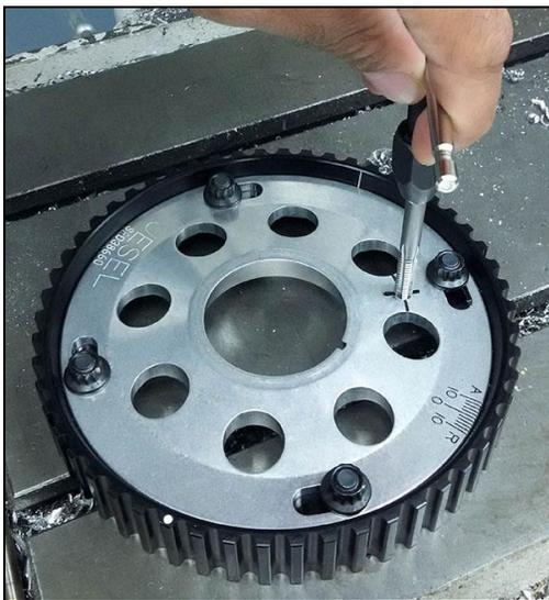
**Figure 12: Tapping the Cam Hub**
