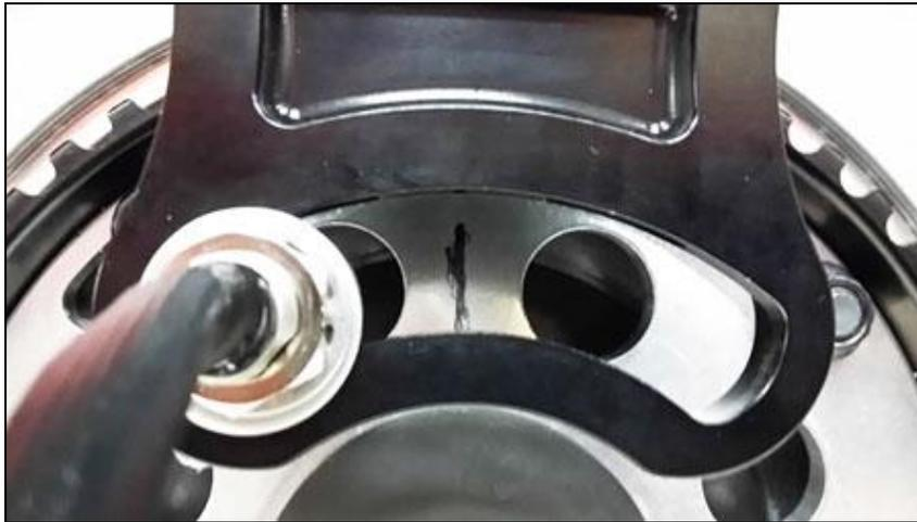
**Figure 9: Angular Reference Marking**
