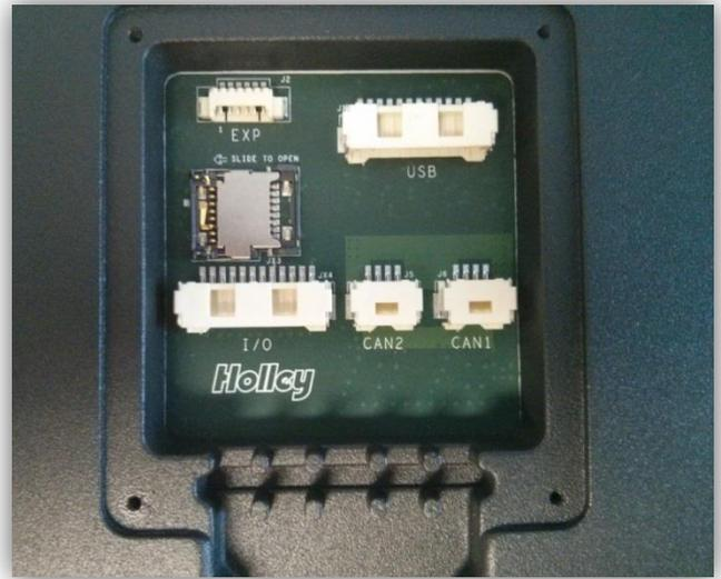
Figure 1. Slide door to the left to unlock
